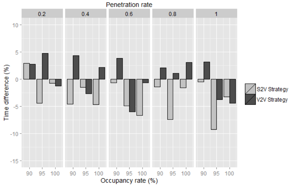
Figure 2. Overall time difference for V2V strategy and S2V strategy, for different occupancy rates and penetration rates, for heterogeneous driver behavior.
